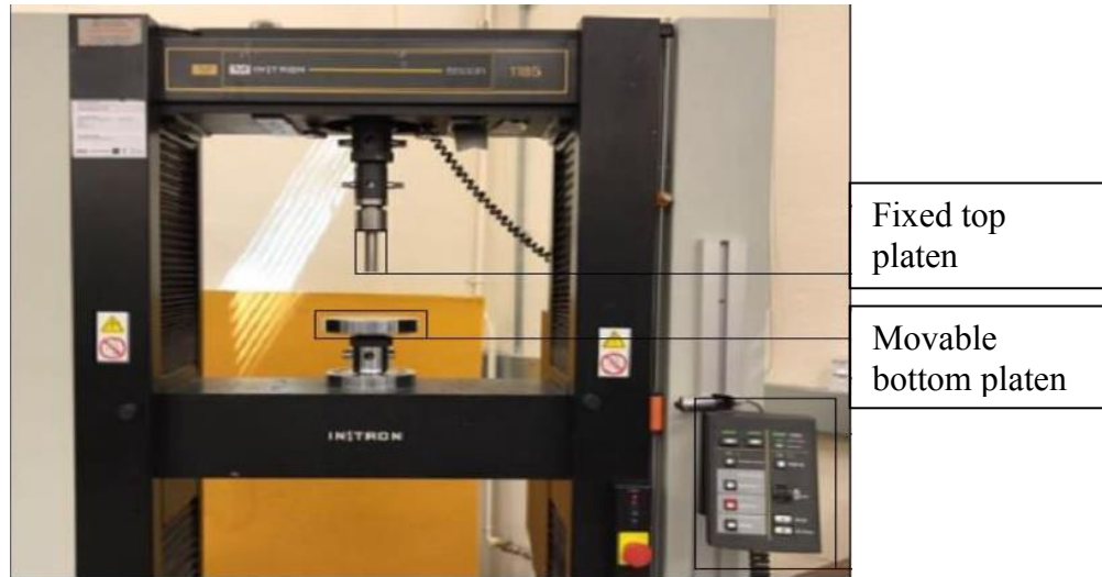
Fig. 5.4 Uniaxial compression testing machine
