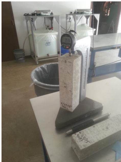
Figure 3-14. ASR prism being tested for expansion.
