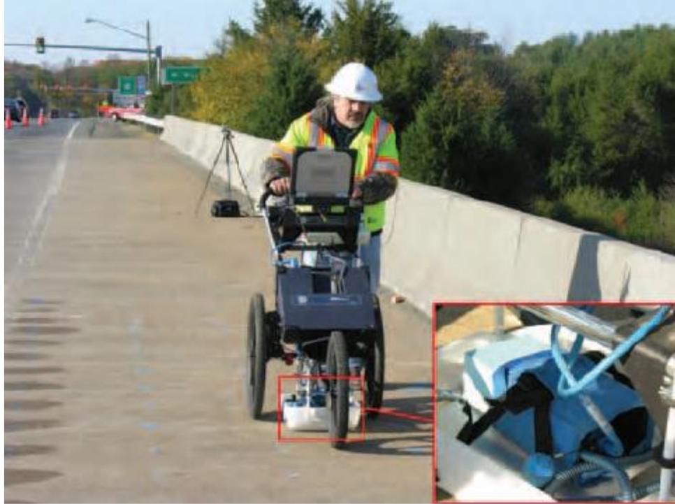
Figure 2-3. Ground Penetrating Radar (GPR) (Gucunski 2013. Used with permission).
