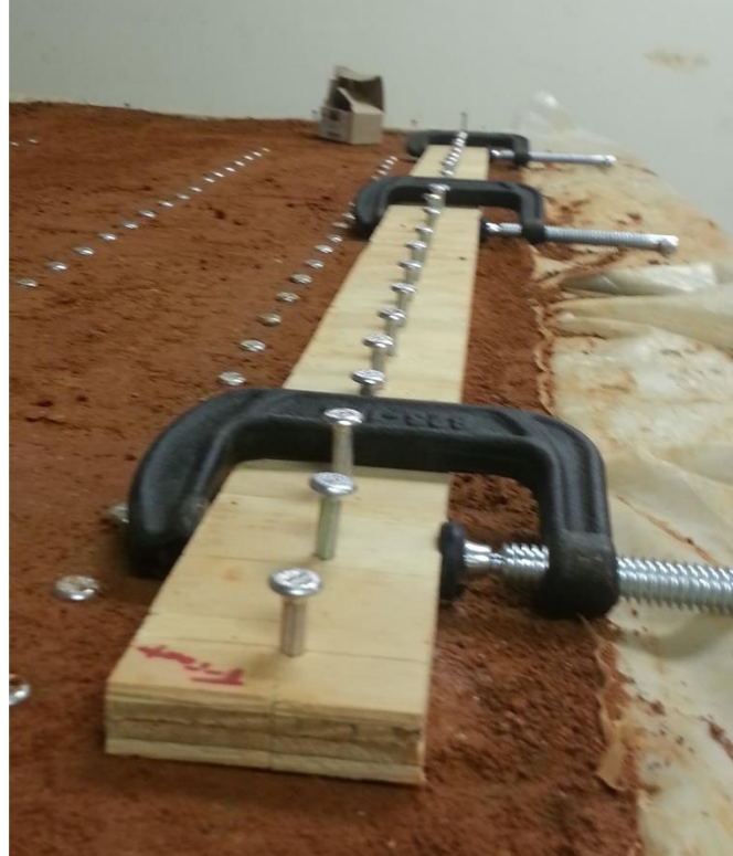
Figure 3-5. Template for placing masonry nails in soil.
