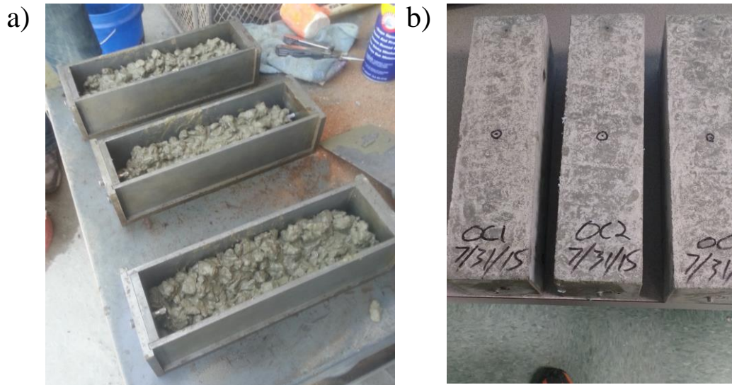
Figure 3-11. a) Casting of prisms and b) cured prisms.
