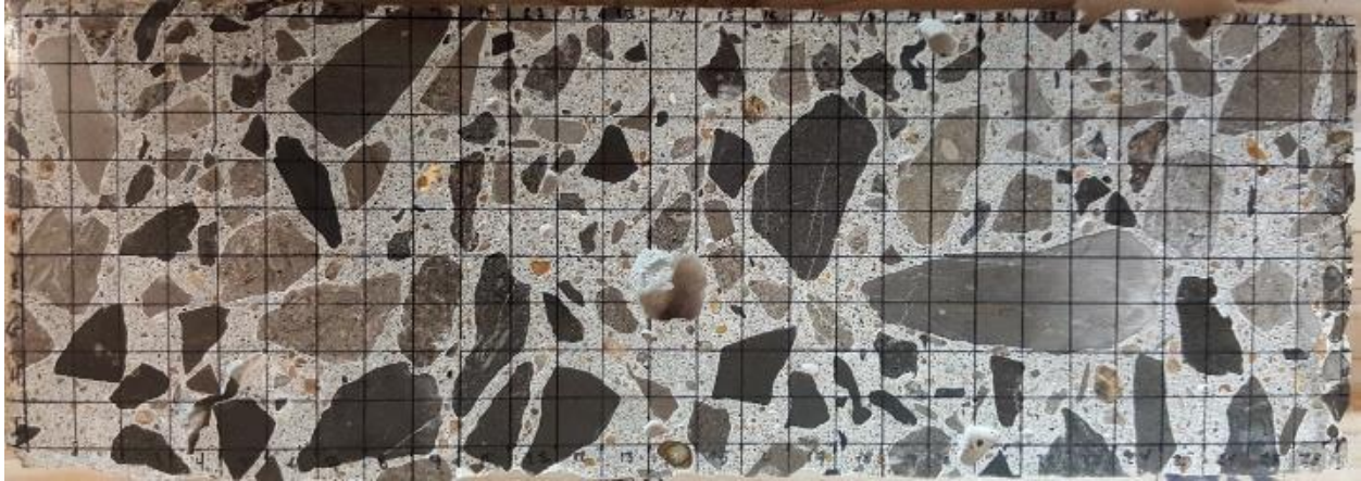
Fig. 4.3-3 —Typical DRI sample with reference grid (by Richard Deschenes Jr.).
