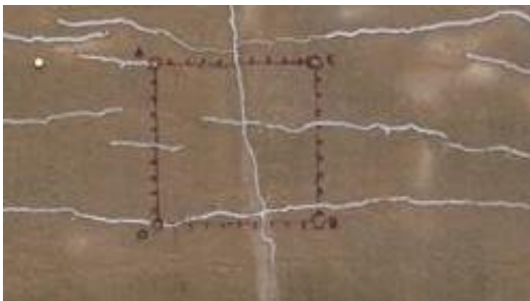
Fig. 3.3-3 —Typical strain measurement grid on barrier section after treatment with silane (by Richard Deschenes Jr.).
