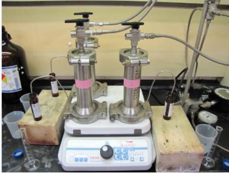
Figure 3-8: Membrane Bench Test Apparatus – As Tested
