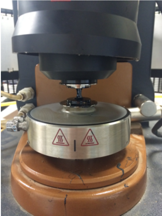
FIGURE 2. Determination of Rheological Properties of Asphalt Emulsion using DSR (Photo taken by S. Smith)
