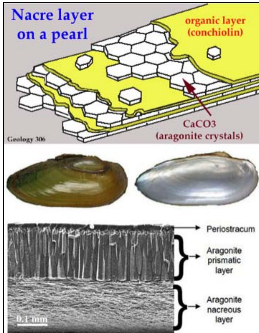
Figure 2.2 Schematic and scanning electron microscope images of the structural arrangement for aragonite crystal layers found in nacre (Meyers, Chen, Lin, and Seki, 2008).
