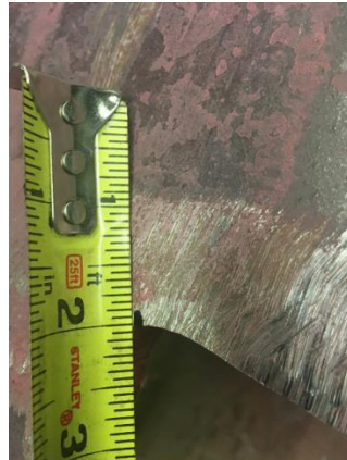
Figure 50. Notch at weld corner (8 million cycles)
