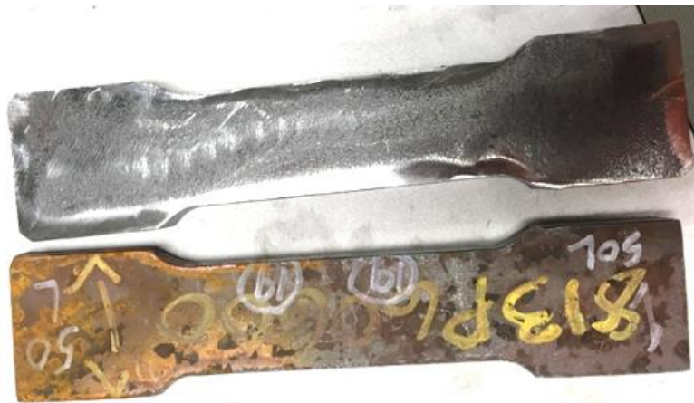
Figure 31. Corroded (bottom) and uncorroded (top) steel surfaces
