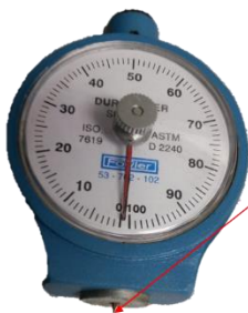
Shore D Durometer Hardness measuring device.
