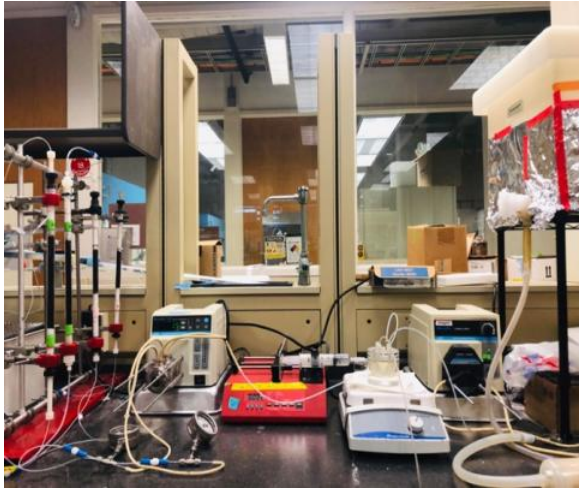
Figure 2-1. Photographs of packed-bed columns. The left-side photo shows lab-scale RSSCT setup including a feedwater tank, inline filter, peristaltic pumps, mixing jug, stirrer, syringe pump, and glass columns filled with GAC. The right-side photo shows glass columns filled with GAC in a packed-bed set using plungers and glass wool.
