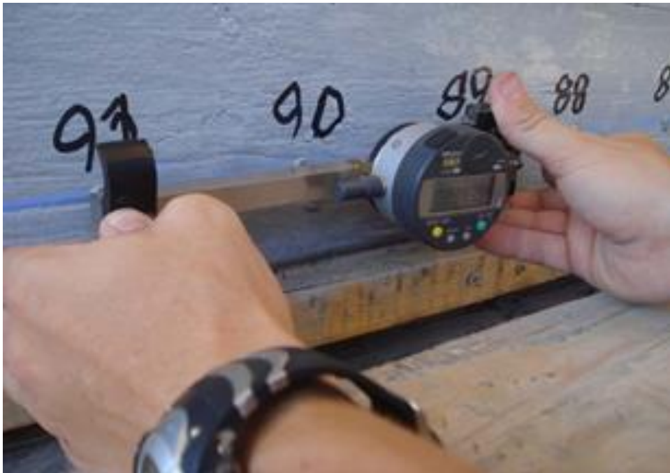
Figure 2-3. DEMEC measurements (Photo by author).
