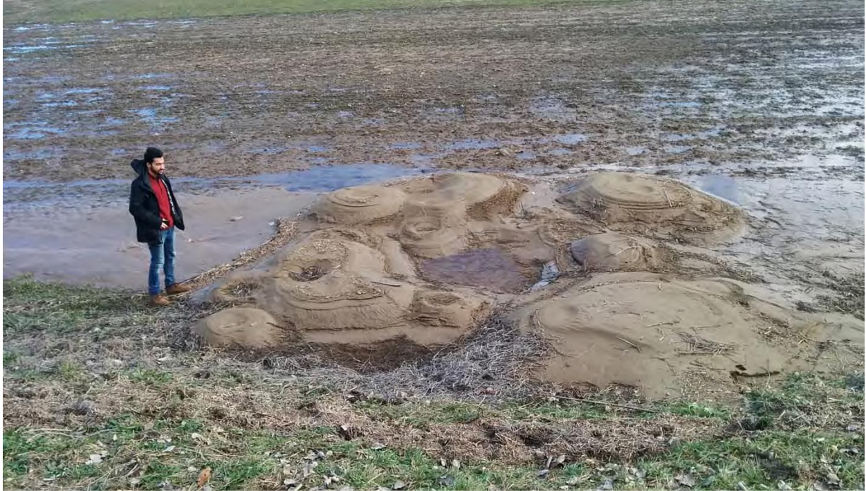
Figure 7 - Large sand boil network at levee toe near Olive Branch, IL (Rutherford et al., 2016)
