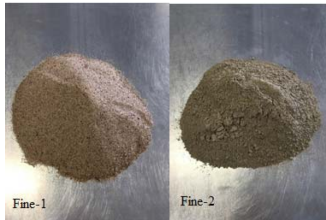
Figure 3-2. Two types of fine materials used in the experimental program. Fine-1 is Arkansas River sand, and Fine-2 is Class C fly ash
