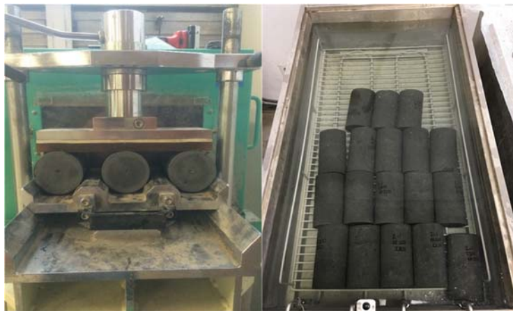
Figure 2-5. End-grinder and water bath used for heat curing
