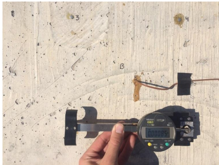
Figure 3.4 – Expansion/strain measurement with DEMEC gauge
