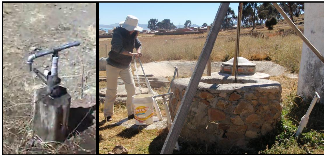
Figure 4-2. (a) Photo of EMAS Flexi-Pump on manually drilled well [left]; (b) Photo of multiple EMAS Pumps installed on a single hand-dug well [right]
