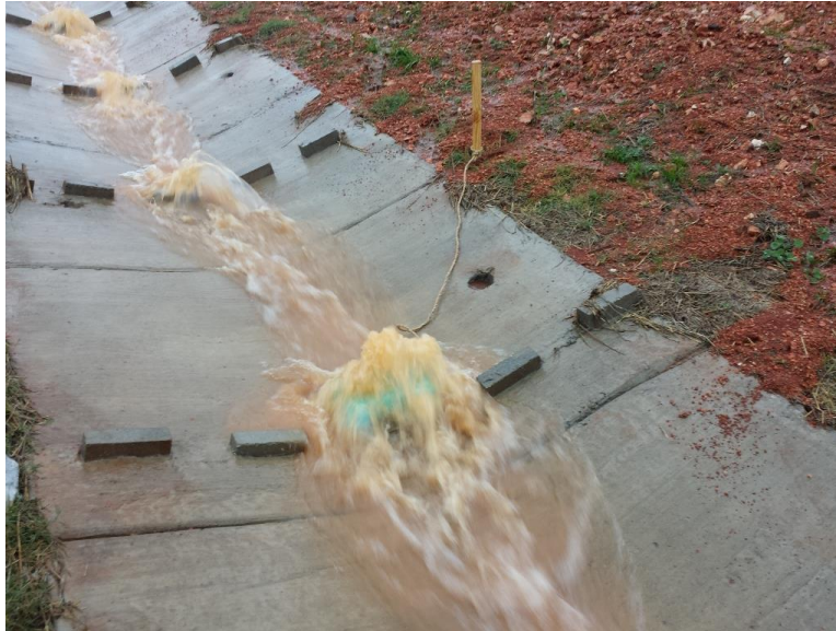
Figure 3.3: A stream inflow where a 703d#3 Floc Log was placed on a concrete ditch. Photo taken by author.
