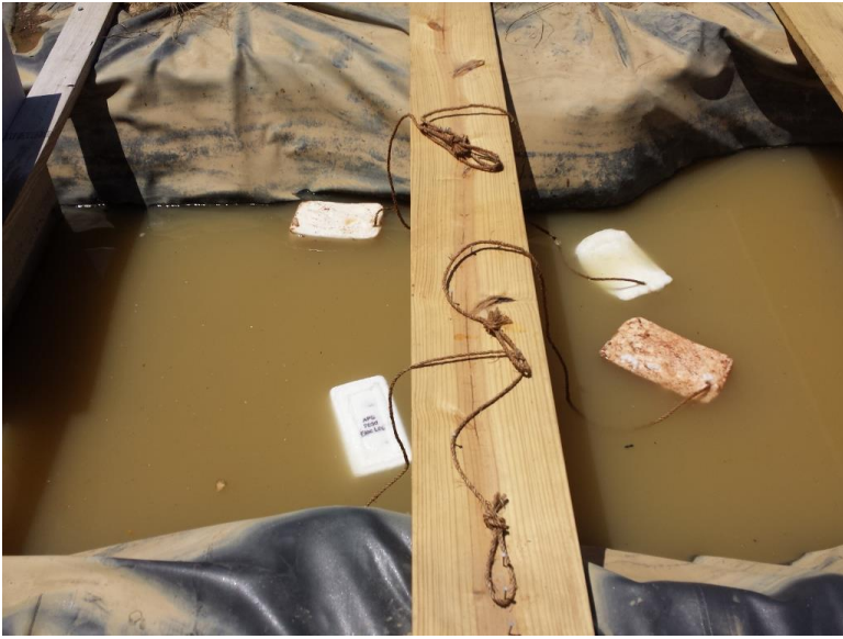
Figure 2.4: Photograph of four 703d type Floc Logs suspended in the turbidity test channel. Photo taken by author.
