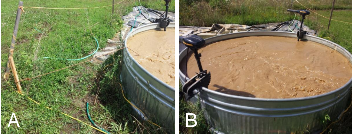
Figure 2.5: Photographs of the basin-scale jar tests. (A) Photo of the Floc Log roped around a stake and suspended in the turbid water tank, (B) Photo of the stock tank filled with turbid water with the two trolling motors attached. Photos taken by author.
