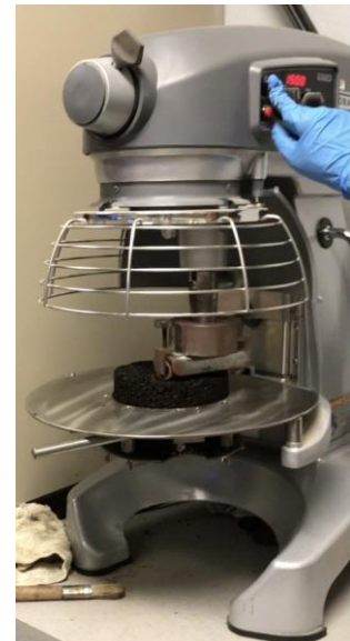
Figure 16. Hobart mixer for raveling test
