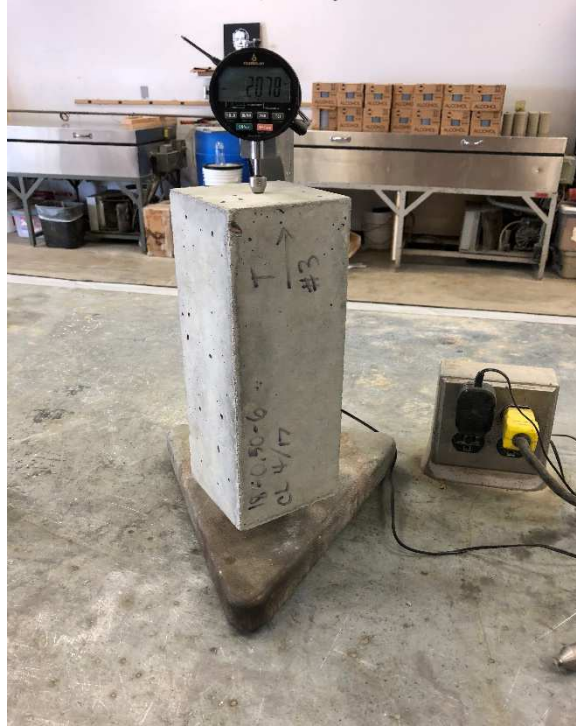
Figure 3.4. Shrinkage Prism Testing
