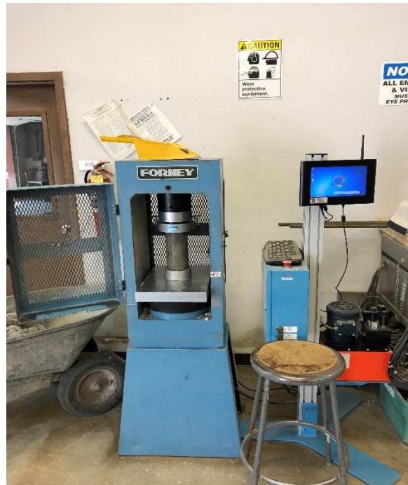
Figure 3.3. Compressive Strength Testing
