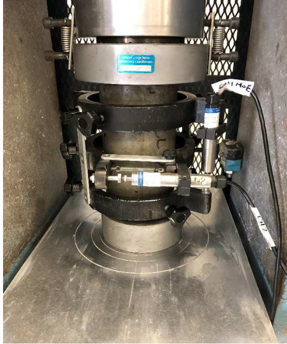
Figure 3.5. Modulus of Elasticity testing
