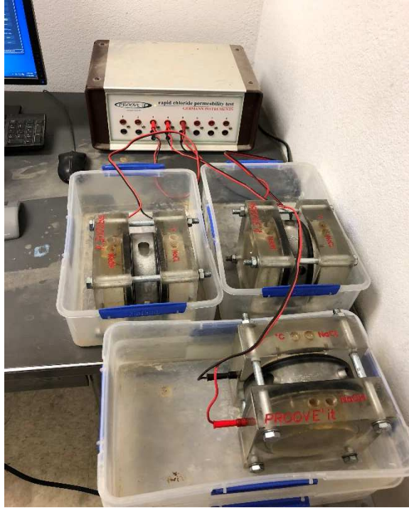
Figure 3.6. Rapid Chloride Ion Permeability testing
