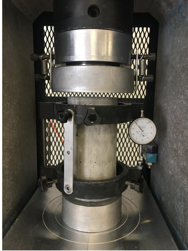
Figure 3.5. Modulus of elasticity setup using Forney
