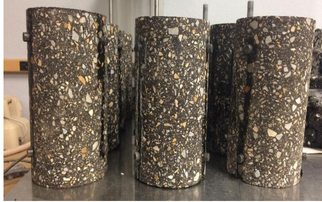
Figure 6. Uniaxial |E^*| Geometry
