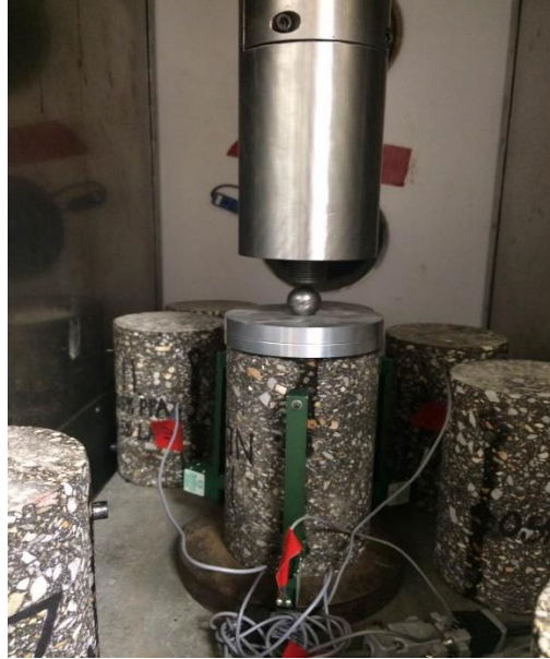
Figure 9. Uniaxial |E^*| Test
