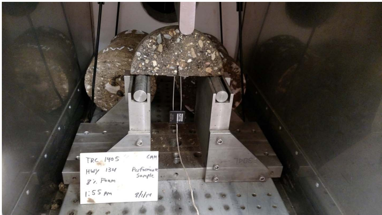
Figure 2.5.2.1 – Semi-Circular Bend Test Configuration (Photo Credit – Chase Henrichs)
