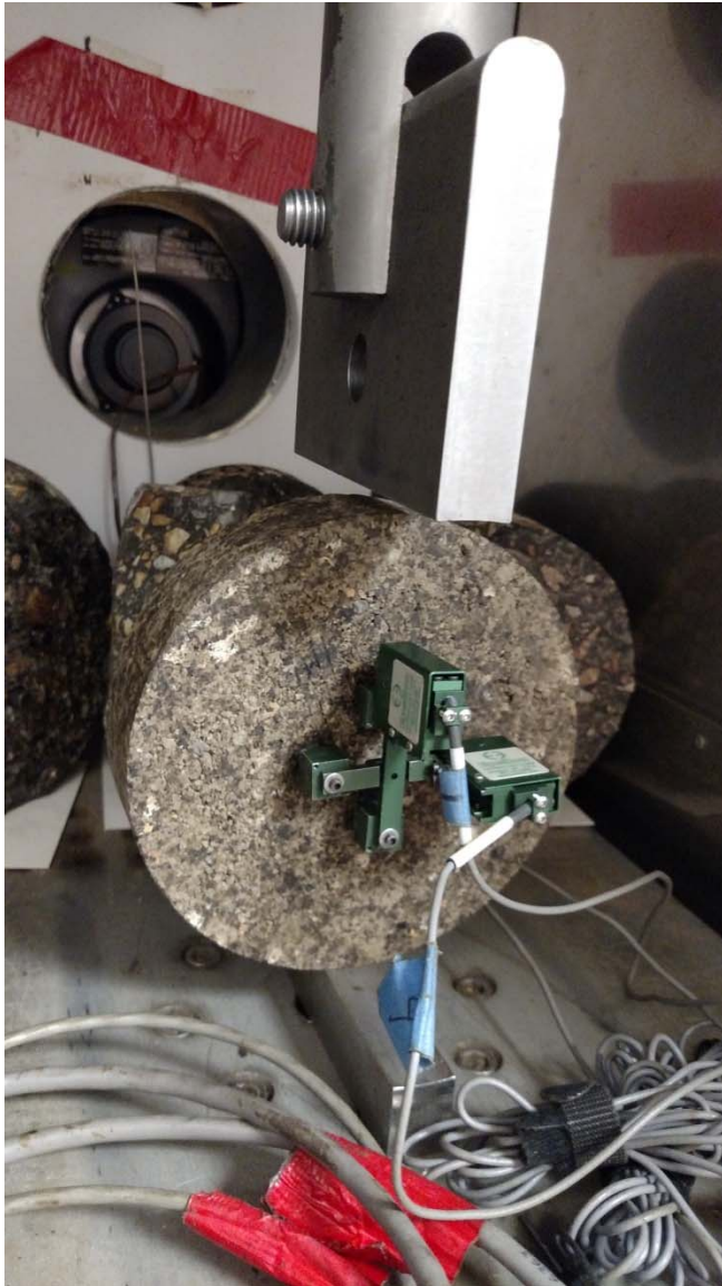
Figure 2.5.1.1 – Dynamic Modulus and Creep Compliance Testing Configuration (Photo Credit – Chase Henrichs)
