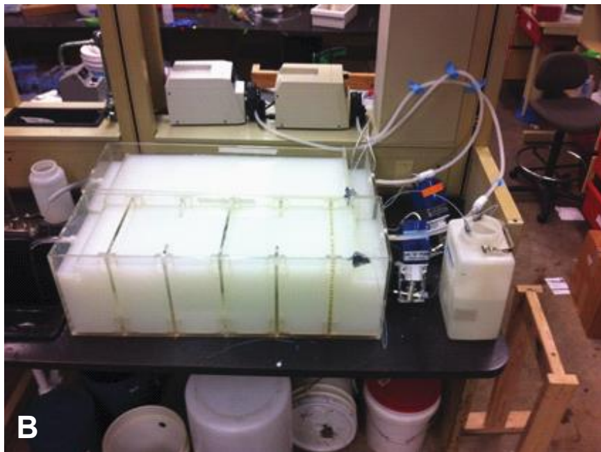
Figure 2.1: Photographs of the Phase II lab-scale hydraulic flocculation setup. (A) a 200 L bucket filled with tap water amended with 2 \text{ g L}^{-1} kaolinite mixed at constant speed with a paddle controlled by a drill, (B) two 65 L flow through reactors (baffled reactor in the foreground), two peristaltic pumps (in the background) to supply the turbid water to the reactors, and a 9 L carboy containing PAM stock solution supplied to the reactors with a piston pump (to the right of the reactors), and (C) effluent of the two 65 L reactors. Photos taken by the author.
