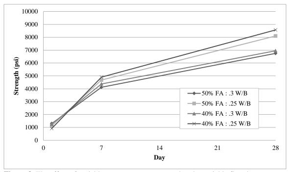
Figure 8. The effect of variable water content compared to the variable fly ash content
