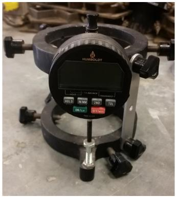
**Figure 3**. Modulus of elasticity testing collar
