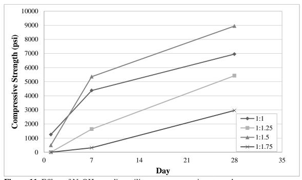
Figure 11. Effect of NaOH to sodium silicate on compressive strength
