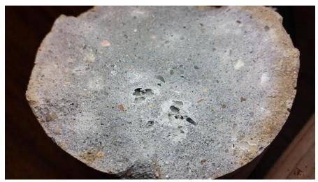
Figure 7. Undissolved chemicals in the mortar
