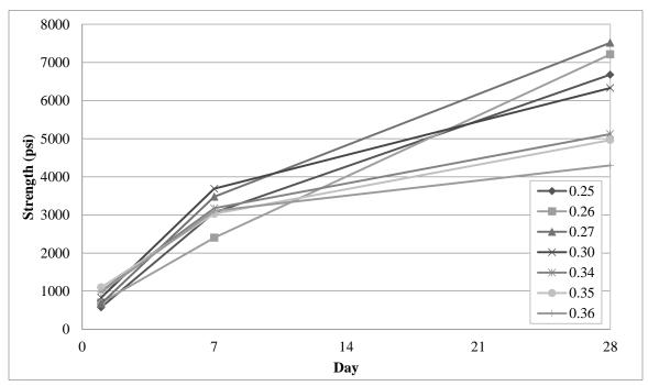
Figure 4. Compressive strength at 1, 7, and 28 Days as a result of water to binder ratio
