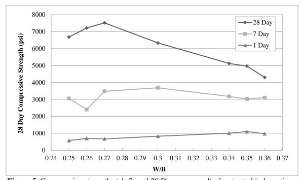
Figure 5. Compressive strength at 1, 7, and 28 Days as a result of water to binder ratio
