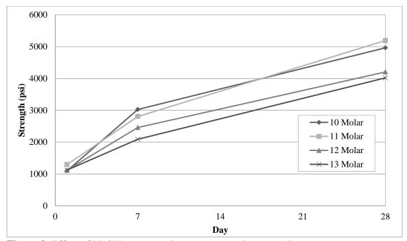
Figure 9. Effect of NaOH concentration on compressive strength
