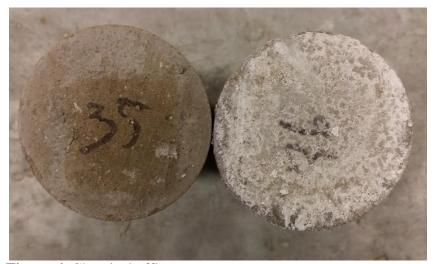
Figure 6. Chemical efflorescence
