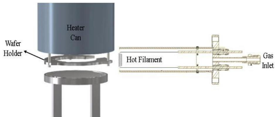
Figure 8.1: Schematic diagram of the hot-filament design in the UHV-CVD system.
