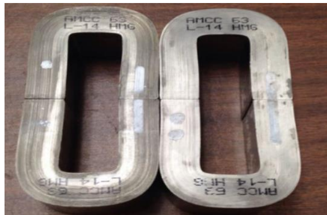
Figure 4.5. Metglas Amorphous AMCC – 63 laminated core.
