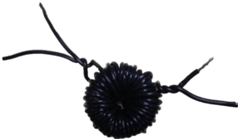
Figure 4.14. The fabricated 100 kHz nanocrystalline toroid transformer.
