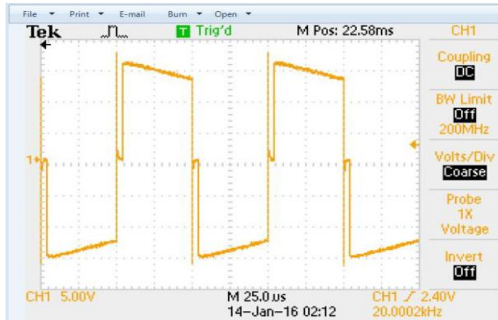
Figure 4.10. Transformer input voltage for V_{in} = 30 V.
