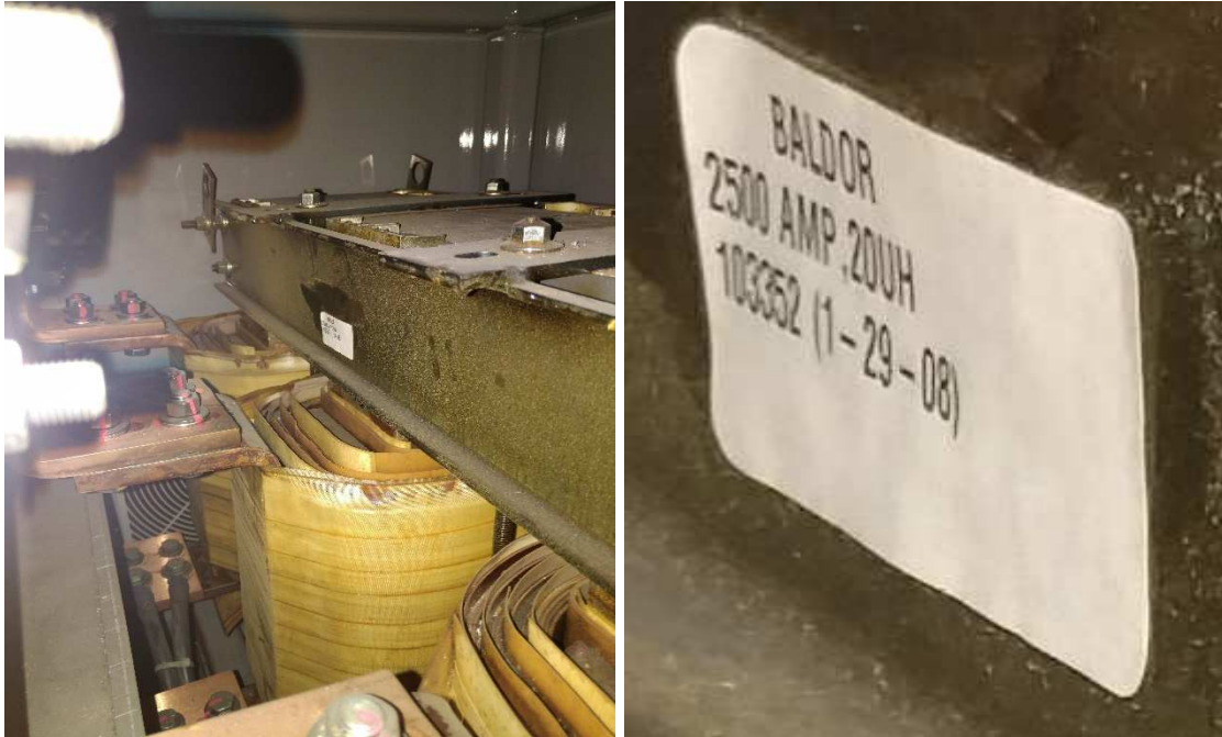
Figure B.3 Filter Inductors in REGEN bench (left) and model of Filter Inductors (right).
