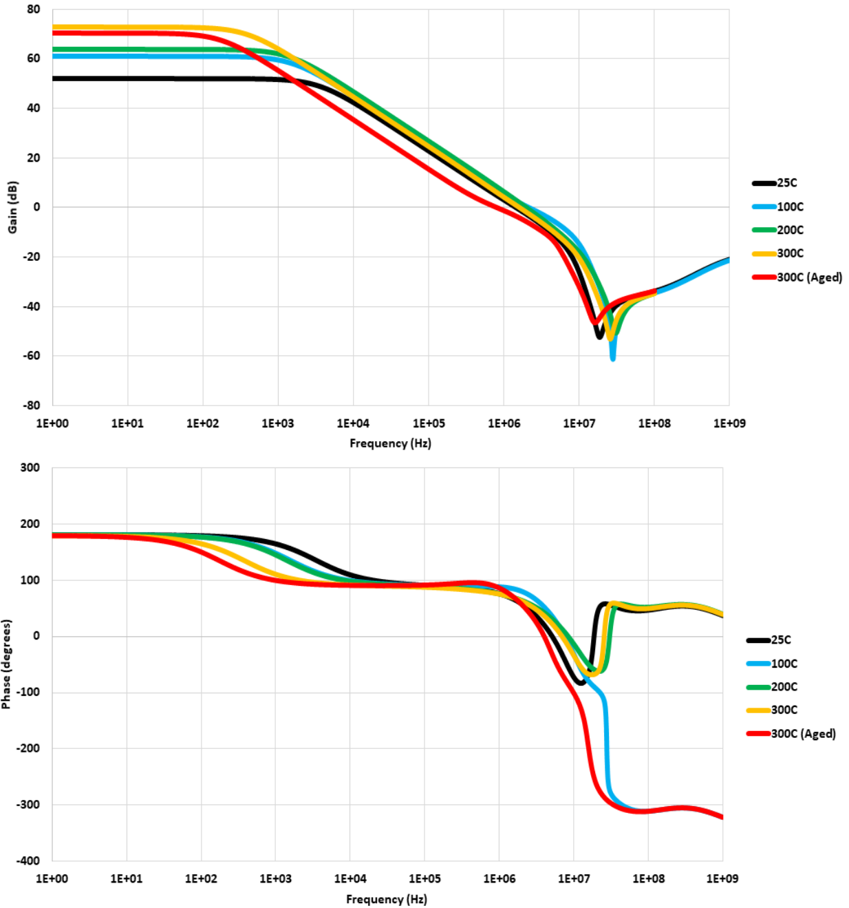
Fig. 4.35. The frequency response of the fully on-chip NFET linear regulator for V_{IN} = 20\text{ V} and I_{LOAD} = 50\text{ mA} across the operating temperature range.
