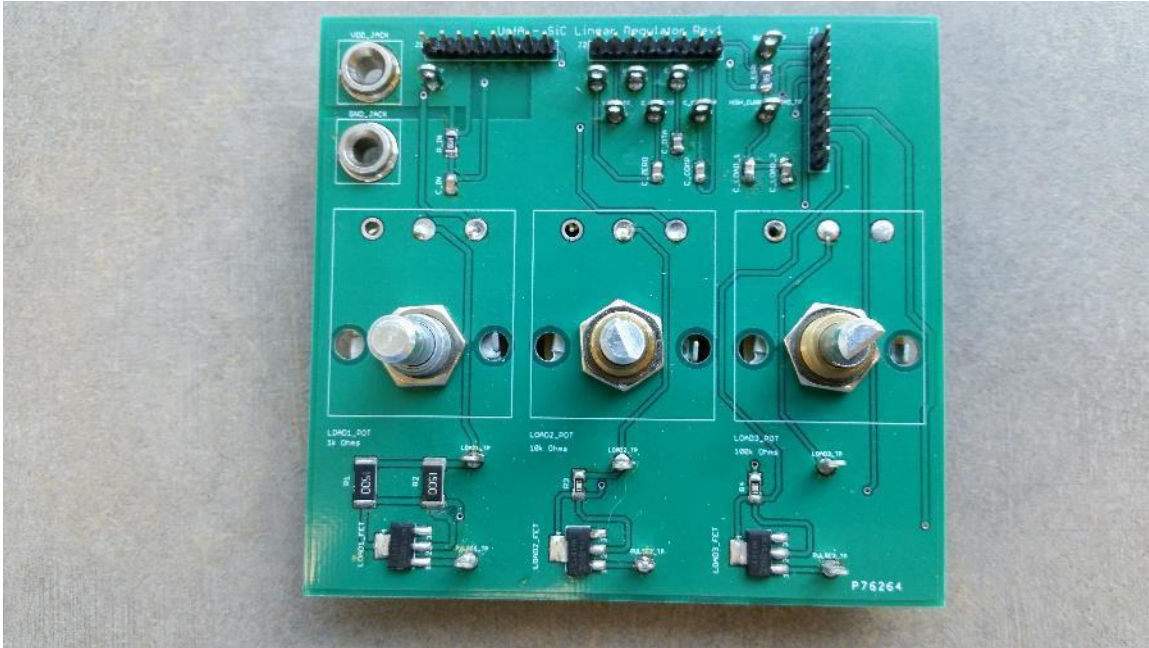
Fig. 5.6. The breakout board created for characterizing the linear regulator.
