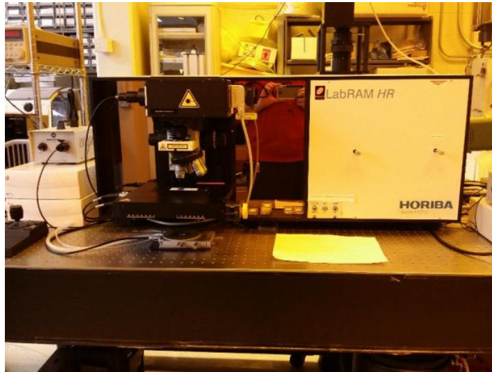
Figure 3.5. HORIBA LabRam HR Micro Raman system. “Photo by Yahia Makableh”
