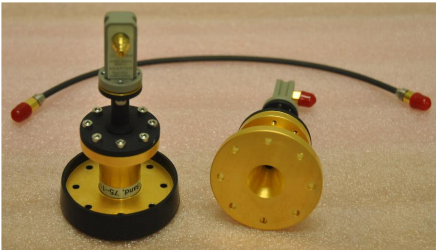
Figure II.13. W-band transitions with 1.00 mm coaxial connectors and 1.00 mm coaxial cable.
