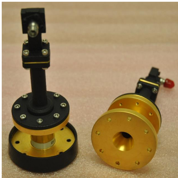
Figure II.10. Ka-band transitions with 1.85 mm coaxial connectors.
