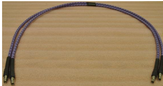
Figure II.5. Air dielectric cables.
