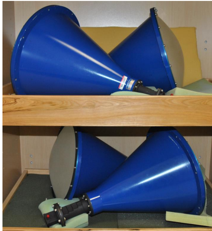
Figure II.19. C-band and X-band horn lens antennas.
