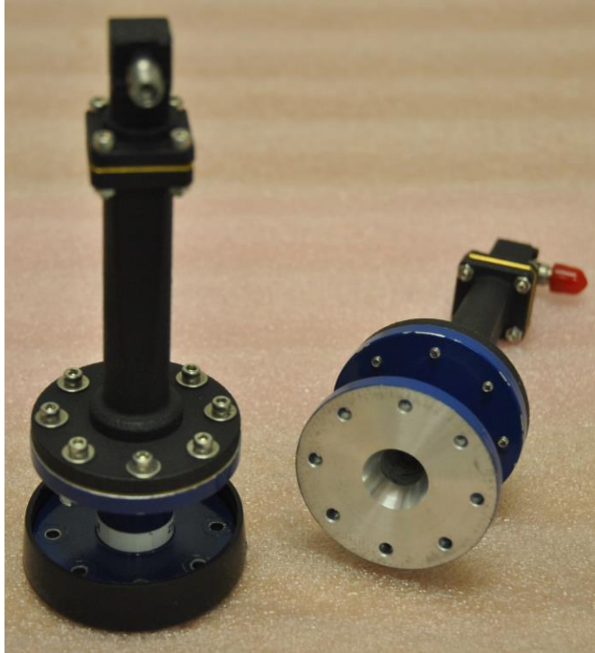
Figure II.9. K-band transitions with 1.85 mm coaxial connectors.
