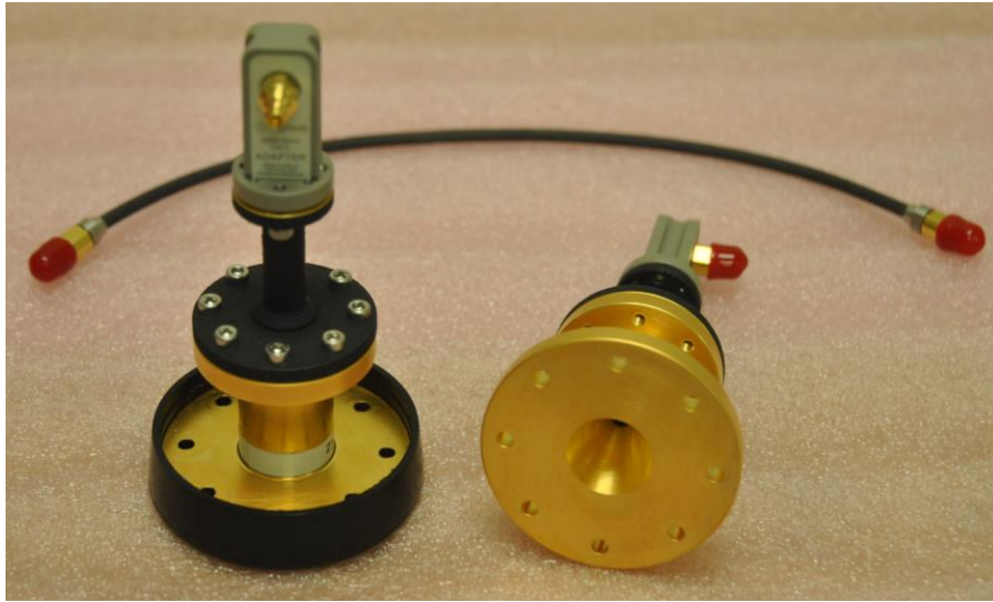
Figure II.12. V-band transitions with 1.00 mm coaxial connectors and 1.00 mm coaxial cable.
