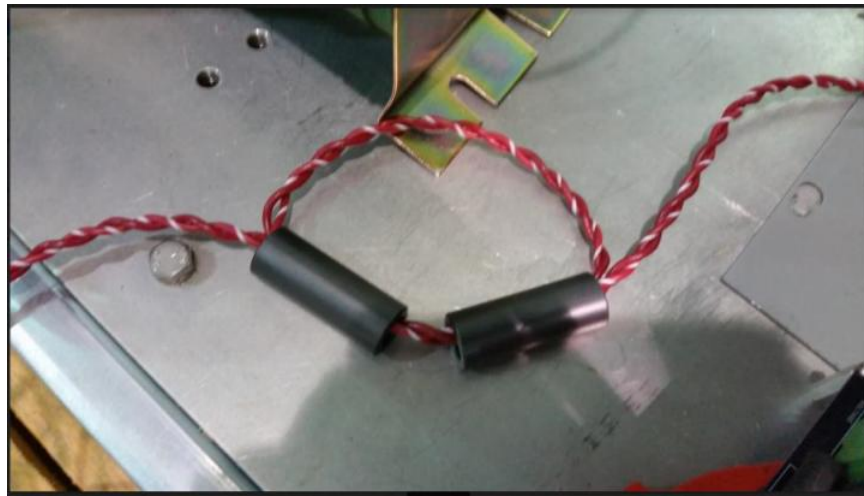
Fig. 6.21 EMI suppression axial ferrite beads for reducing conducted EMI.
