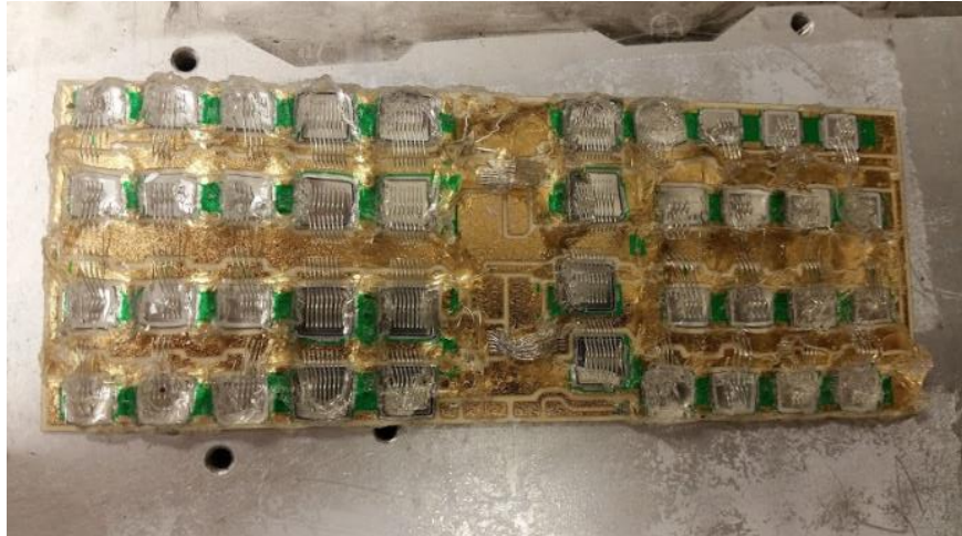
Fig. 6.11 Chips of IGBT and free-wheeling diode of an IGBT module.
