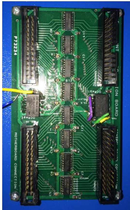
Fig. 3.4.19: Populated Control Isolation Board Picture
