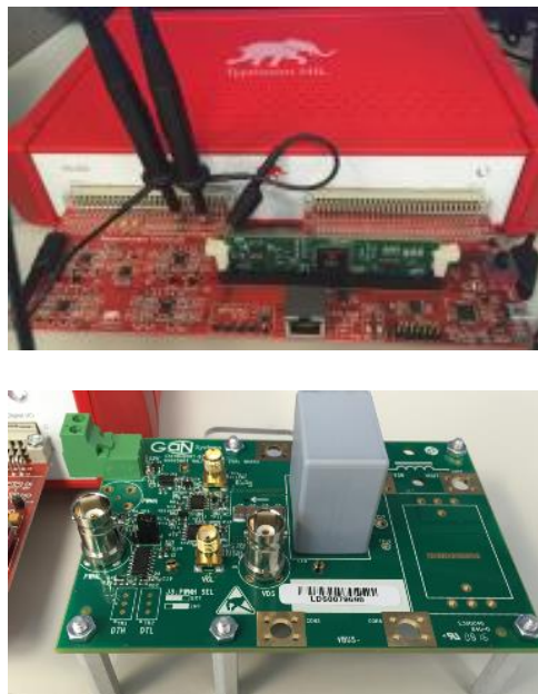
Fig. 2-25 Experimental Setup: Typhoon Simulator and DSP Control Card
