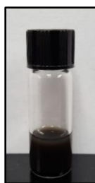
Figure 2.3. Nickel oxide nanoparticles are dispersed in butanol for spin coating application. “Photo by Ramesh Vasam”
