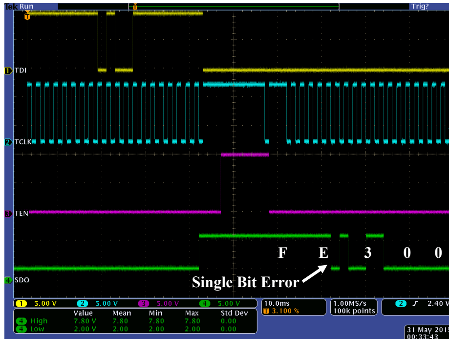
Fig. 6.19 R1C2 gate-source test, with a fault in 6 th bit. The yellow trace is the test data input (TDI), the cyan trace is the test clock (TCLK), and the magenta trace is the test enable input (TEN). The green trace observes the serial data output (SDO) from the gate driver IC. The serial data output reads 0xFD300, which indicates a fault (expected 0xFF300).
