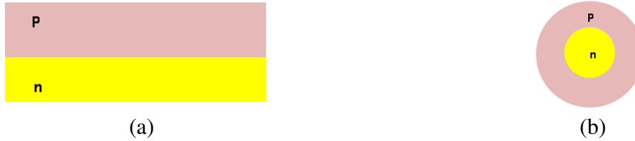
Fig. 6.1. Schematic of PN junctions: (a) Vertical cut plane to flat PN junction PVSC, and (b) Horizontal cut-plane of radial PN junction PVSC.
