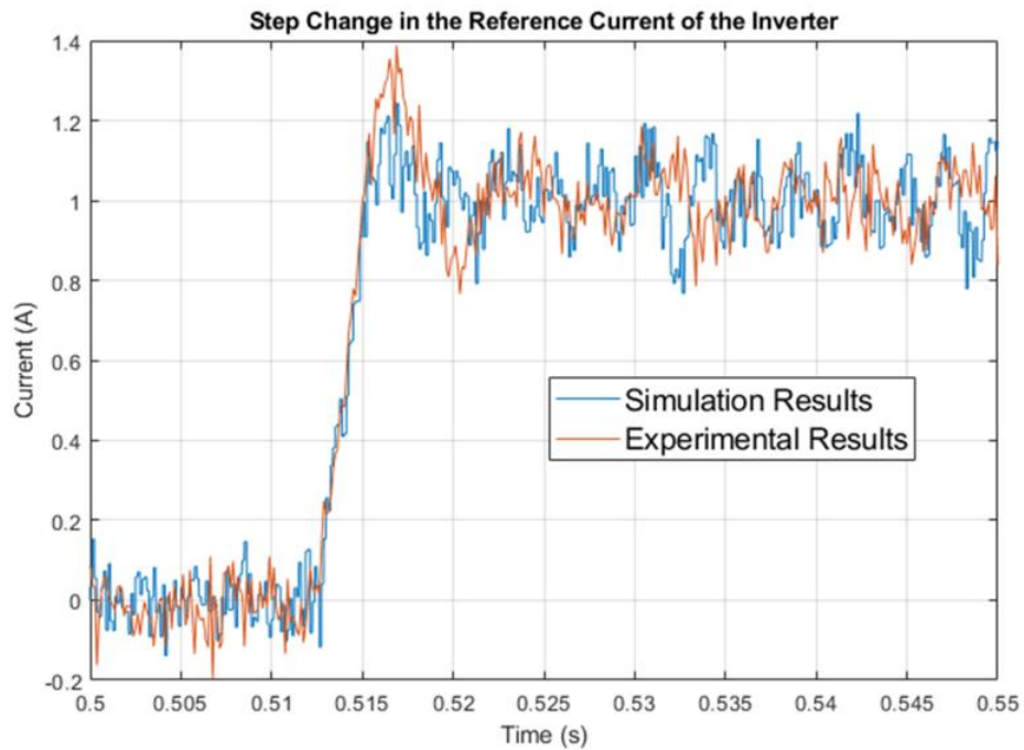
Fig. 6.3: Step change in reference current of the inverter.
