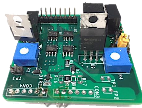
Figure 5.5. ML gate driver board.
