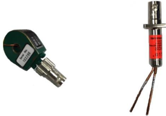
Figure 5.1. Pearson current monitor and coaxial shunt current viewing resistor.
