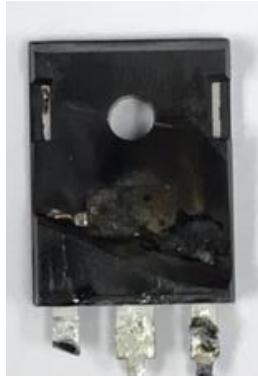
Figure 2.5. Failed SiC MOSFET due to short circuit.
