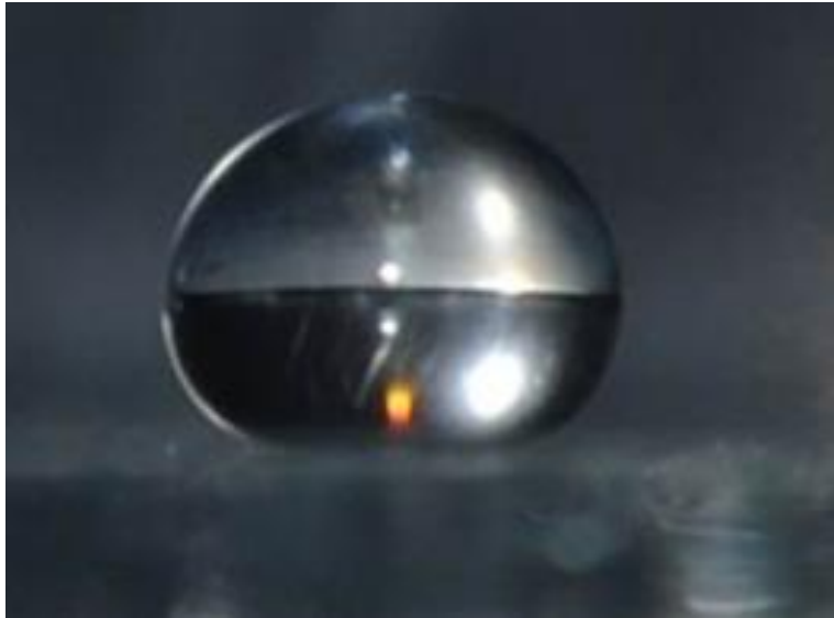
Figure 3.12 A water droplet sits on a silica base hydrophobic surface
