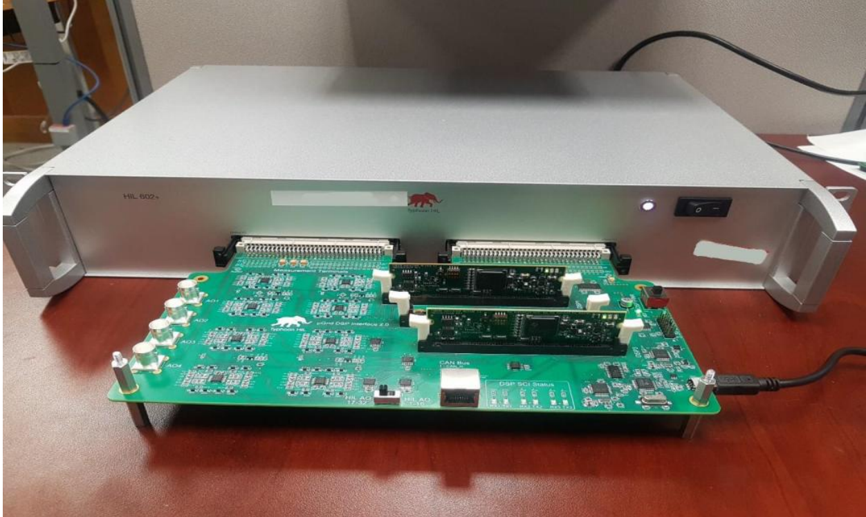
Figure 5.1: Typhoon HIL setup for controller HIL testing
