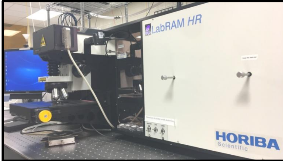
Figure 1. 9 Snap shot of the LabRAM HR Evolution – Horiba Raman-PL microscope in the lab.
