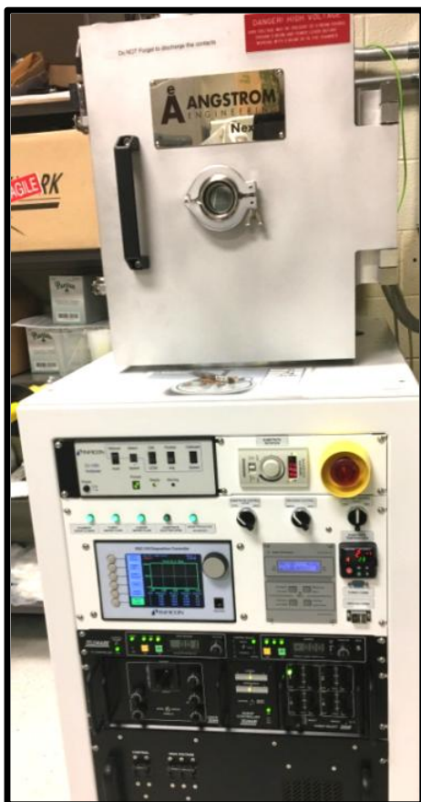
Figure 1.10 Snap shot of the Angstrom Nexdep Electron Beam Evaporator in the lab.
