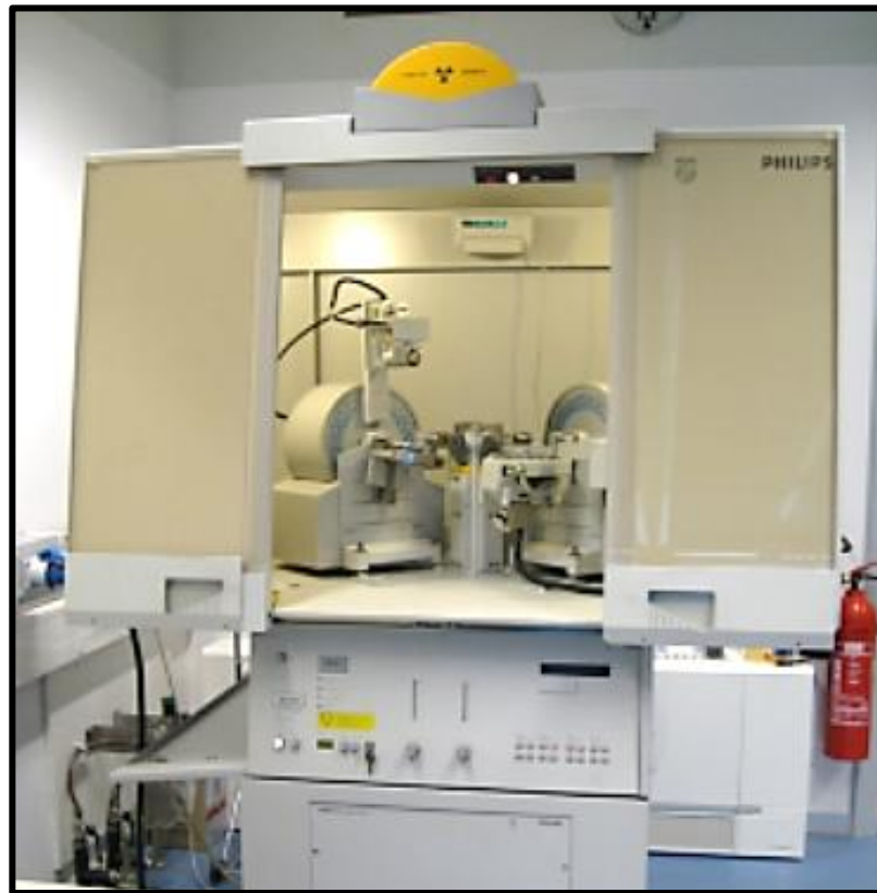
Figure 1. 4 Philips PW-3040 XPert MRD High Resolution X-Ray Diffractometer [39]
