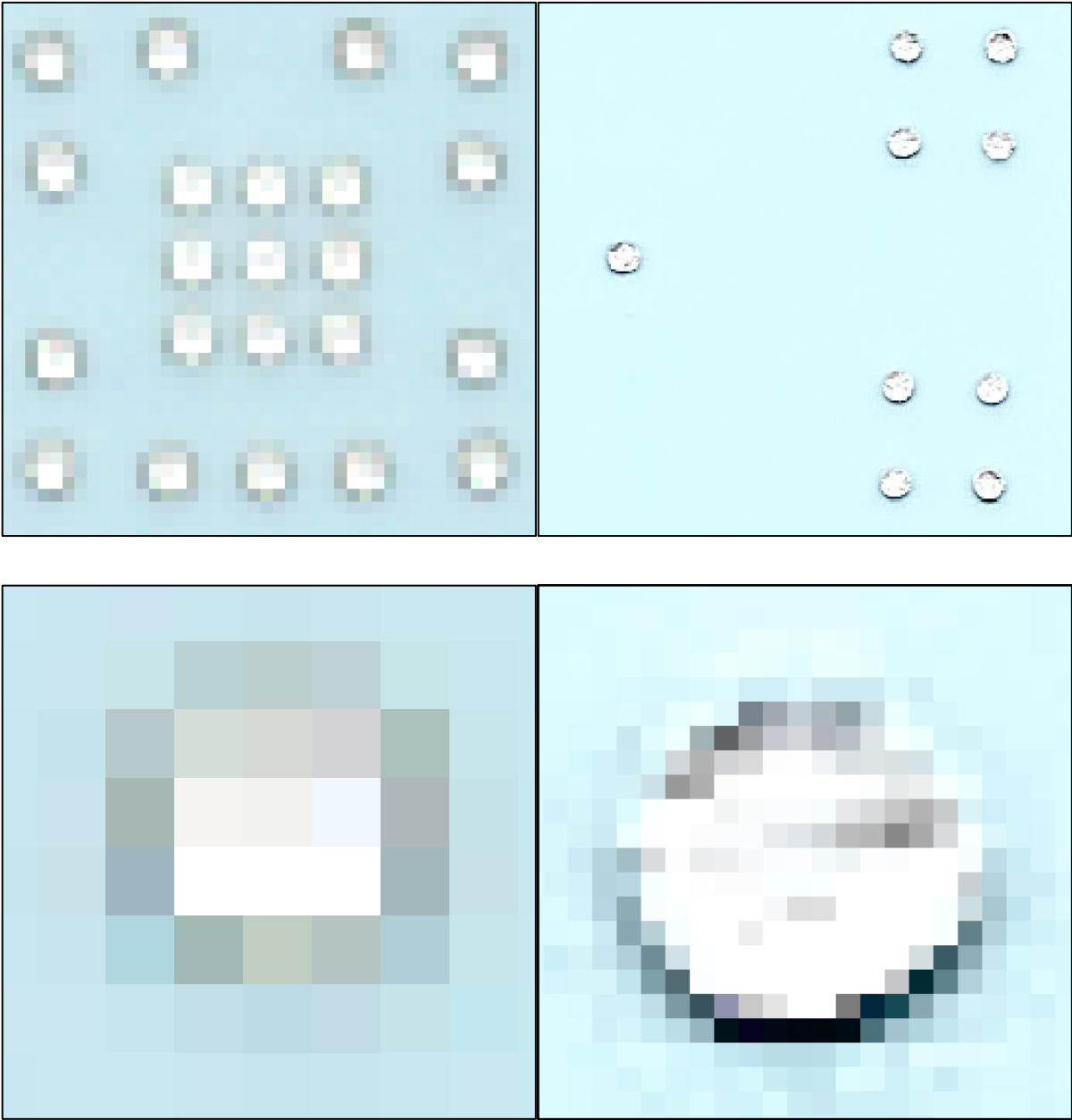
Fig. 4.5. (top left) Zoomed in image of 600dpi via structure (top right) zoomed image of 1200dpi via structure (bottom left) single via in 600dpi (bottom right) single via in 1200 dpi
