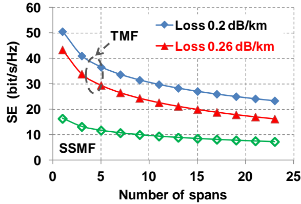
Figure 2.9. Spectral efficiency (SE) for TMF systems. SE of SSMF is also drawn for comparison.
