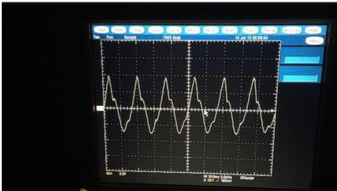
Figure 6.2: Oscilloscope SpO2 Waveform signal-2 from the developed prototype
