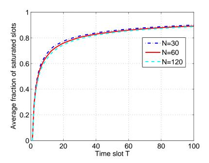
Figure 4.4: The sample average fraction of saturated time slots as a function of time index T. The energy harvesting rate  $\lambda_i = 1/3, \forall i$ , and the network sizes N = 30, 60, 120, respectively.
