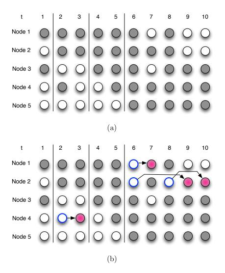
Figure 4.1: Dots represent active sensors in each time slot under the initial scheduling and final scheduling in Fig. 4.1(a) and Fig. 4.1(b), respectively. Arrows connecting a circle and a dot in Fig. 4.1(b) indicates the scheduling adjustments upon the initialization.
