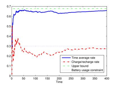
Figure 5.3: A sample path of the time-average transmit rate and the battery charge/discharge rate.
