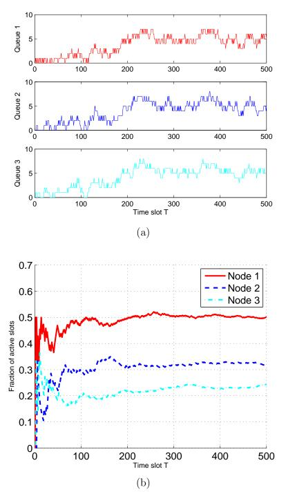
Figure 4.2: A sensor network with N=3,  $\lambda_1=1/2$ ,  $\lambda_2=1/3$ ,  $\lambda_3=1/4$ . Fig. 4.2(a) plots a sample path of the energy queue lengths. Fig. 4.2(b) shows the corresponding fraction of active time slots for each sensor as a function of T.
