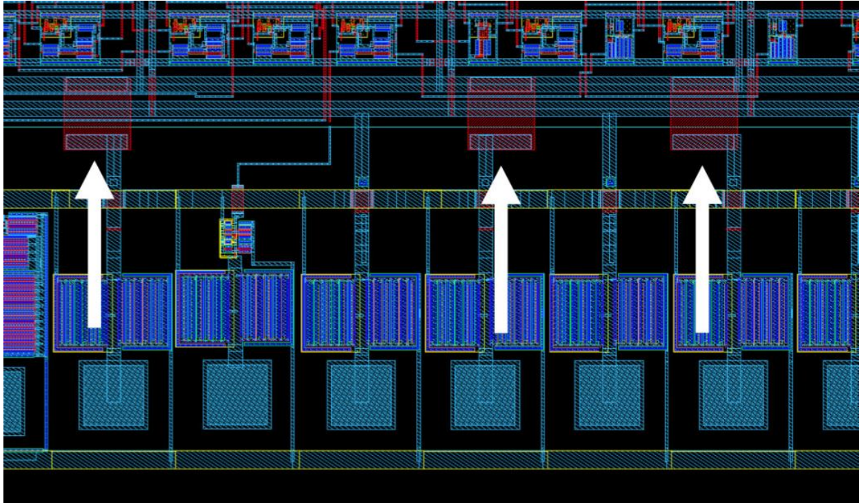
Figure 13. POLY Crossovers in Pad Ring
