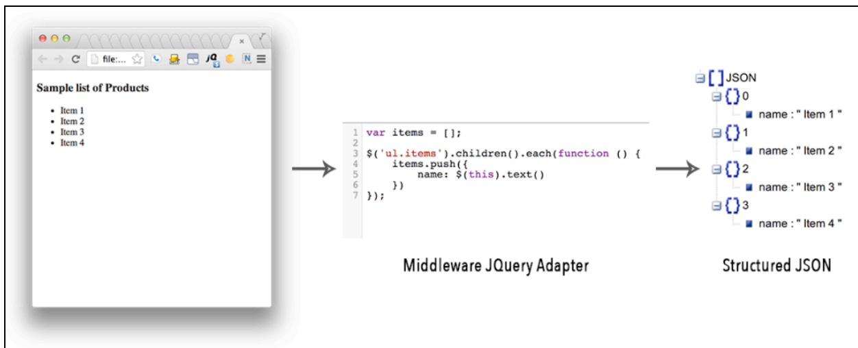
Figure 7: A Simple JQuery adapter to convert a HTML list into structured data
