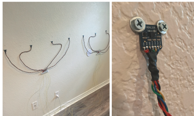
Fig. 24: Experimental Setup for Modeling Vibration Dissipation
