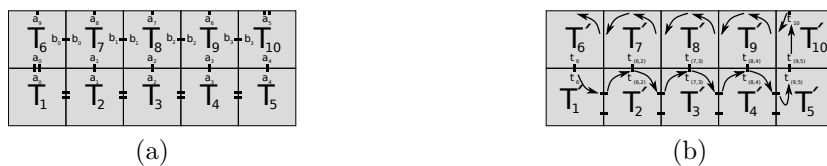
Figure 8.6: (a) depicts zig-zag growth for \tau = 2 . With tiles T_1 through T_5 in place, tiles T_6 through T_{10} must be placed in that order. Moreover, tile T_6 depends only on T_1 , while tiles T_i for i \in \{7, 8, 9, 10\} depend on T_{i-1} and T_{i-5} . (b) depicts zig-zag growth for \tau = 1 using active tiles. Again, with tiles T'_1 through T'_5 in place, tiles T'_6 through T'_{10} must be placed in that order. Moreover, tile T'_6 depends only on T'_1 , while tiles T'_i for i \in \{7, 8, 9, 10\} depend on T'_{i-1} and T'_{i-5} . Also, tiles in each consecutive row contain signals that allow for another row to grow in a zig-zag pattern. Note that only the signals which activate glues which are eventually bound to are shown, while the tiles would actually need to accommodate glues and signals which could represent all possible pairs of input glues for the next growth location.
