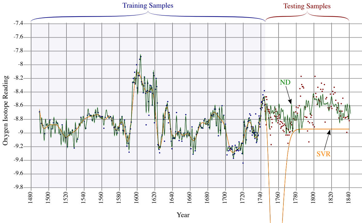
Figure 5.4: A comparison of two predictive models on a series of oxygen isotope readings in speleothems in India from 1489 AD to 1839 AD [32]. Blue points represent the 250 training samples from July 1489 to April 1744 and red points represent the 132 testing samples from August 1744 to December 1839. Because this time-series is irregularly sampled (the time step between samples is not constant), only SVR and ND could be applied to it. SVR, shown in orange, does not perform well, but predicts a steep drop in value that does not occur in the testing data, followed by a flat line. ND, shown in green, performs well, capturing the general shape of the testing samples.
