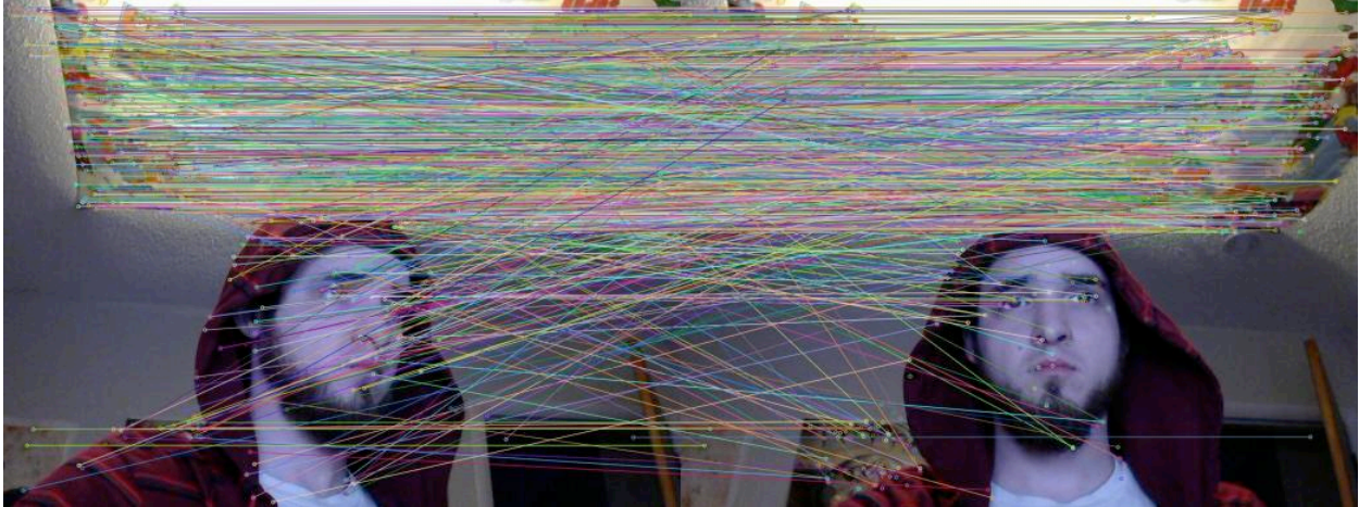
Figure 12: Brute Force SURF Keypoint Matching Output in OpenCV
