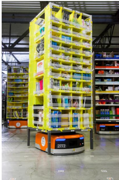
Figure 2.1: Early Kiva Robot by Kiva Systems, Predecessor to the current Amazon Drive Robots, Source: Architects Newspaper [8]
